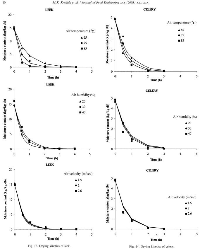
As expected, there is an acceleration of the drying process due to the increase of the temperature of the drying air from 65 to 85 °C. This is very obvious during the first periods of drying. The effect of air
