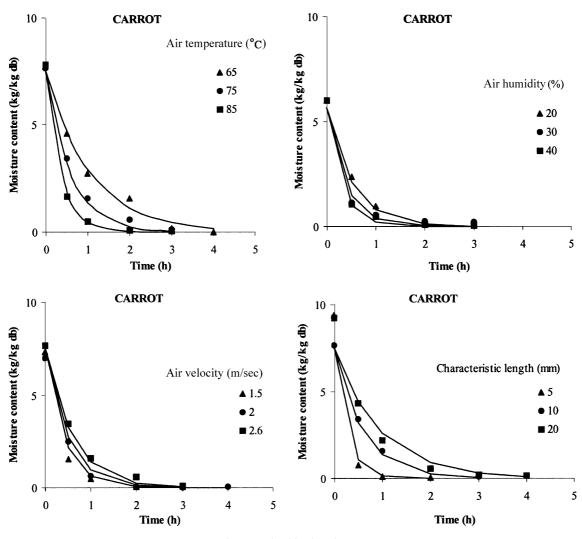
Fig. 6. Drying kinetics of carrot.
