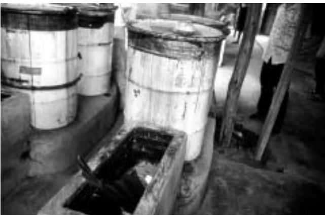
Figure 18. Traditional oil-drum sterilizer
