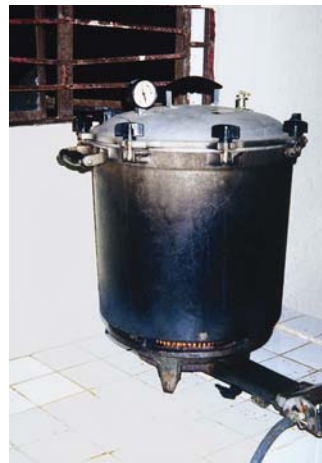
Figure 9. Sterilization at 20 psi for 1 hour
