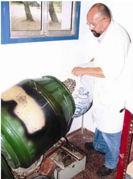
Figure 5. Introduction of sunflower seed hull into drum
