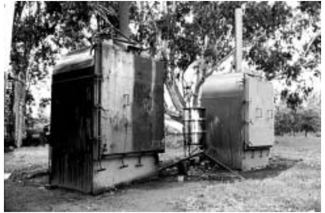
Figure 9. Locally made sterilizers for bags
