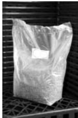
Figure 5. Heat-sealed bags with microfilter windows
