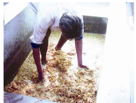
Figure 8, 9. Add soaked wheat straw to the lime stone solution
