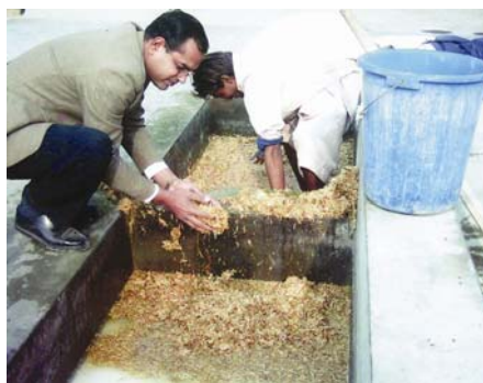
Figure 8, 9. Add soaked wheat straw to the lime stone solution
