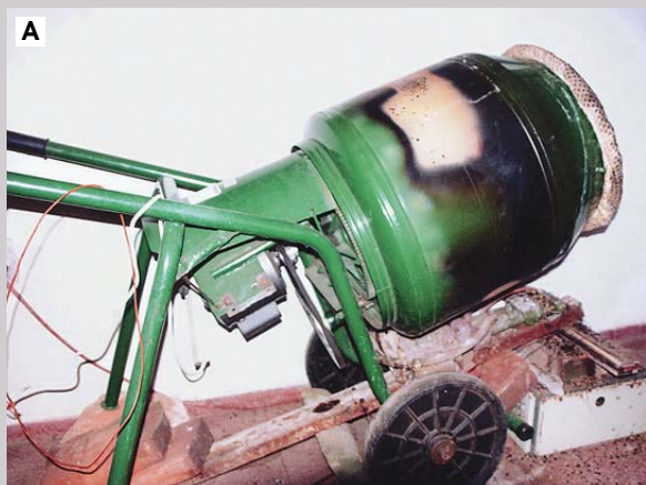
Figure 4. The substrate sterilization and inoculation A: A drum and gas heater for sterilization B: Putting sunflower seed hulls into the drum C: Spawning the decontaminated substrate after cooling D: Filling the bags
